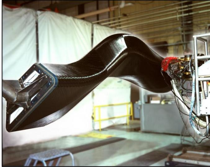
Figure 1. Fiber placement machine building a complex, high performance carbon fiber aircraft engine duct (FP machine on right side). (Photo courtesy of ATK)
